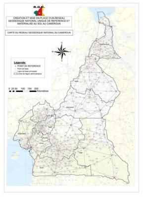
The final geodetic network includes 25 reference stations and 500 network points
