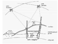
Figure 1: The concept of orthometric height (leveled heights) and ellipsoidal heights (GPS heights) at terrain points with precise geoid heights (Gravimetric/GOCE-derived) about the same adopted reference ellipsoid. (*Source: Johannessen et al*, 2003)
