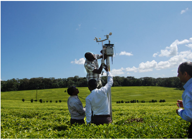
This Wireless Sensor Network (WSN) node was installed on a tea farm in Kericho, Kenya by SERVIR-Eastern and Southern Africa and Kenya Meteorological Services. The WSN supports SERVIR's frost-mapping system by supplementing and verifying satellite data.
